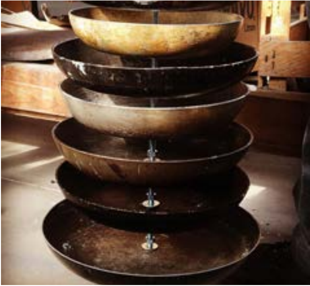
Figure 7. Vertically-mounted pans on a threaded rod, separated by nuts and washers. (In a finished instrument, the nuts will be tightened all the way down.)
