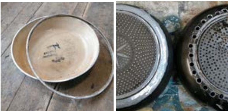
Figure 5. Raise the pitch by removing a slice from the rim. Lower the pitch by grinding on the curve where the side meets the bottom, or by drilling holes around the outside edge.
