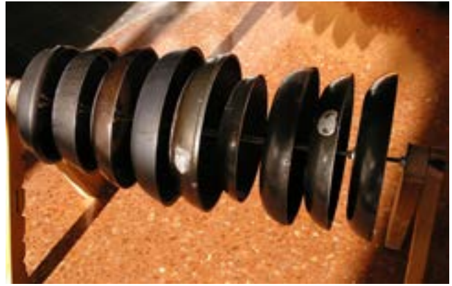
Figure 8. Horizontally-mounted pans on a threaded rod, separated by nuts and washers.
