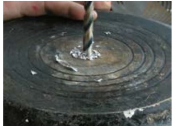
Figure 6. Preparing pans for horizontal or vertical mounting by drilling a hole in the center.
